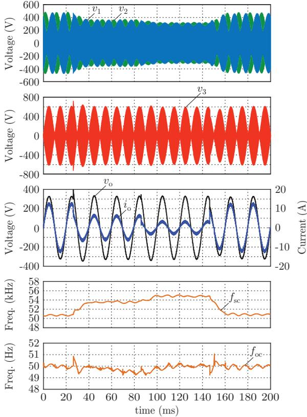
Fig. 8: Transient response simulation results for a 50 % stepwise load reduction after 25 ms followed by another 25 % reduction at 85 ms and a final stepwise increase to the 2 kW rated power at 145 ms, demonstrating the performance of the proposed control strategy.
