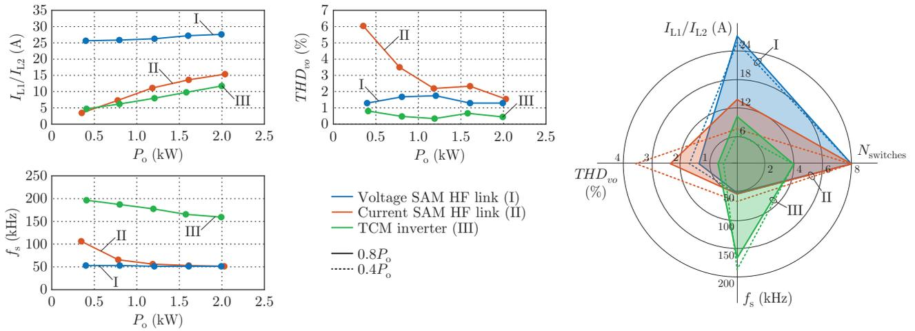
Fig. 9: Performance indicators for comparing both voltage (I) and current (II) SAM HF link converters and the triangular current mode (TCM) inverter (III) [25]. The current-based inverter shows better results regarding tank inductor RMS current values ( $I_{L1}/I_{L2}$ ) which leads to lower conduction losses. In contrast, the voltage-based inverter has lower output voltage total harmonic distortion ( $THD_{vo}$ ).
