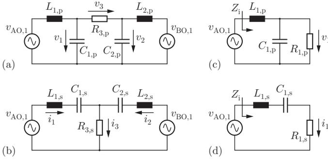
Fig. 3: Simplified circuits that facilitate mathematical analysis and passive component design. Equivalent resistance  $R_{3,p}/R_{3,s}$  represents both cycloconverter and load resistor  $R$ . Circuits in (a) and (b) can be further simplified as shown in (c) and (d) by introducing a time-variant resistance  $R_{1,p}(t)/R_{1,s}(t)$ .
