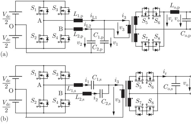
Fig. 2: Voltage- (a) and current-based (b) SAM HF link converter topologies with isolation transformer and center-tapped cycloconverter.
