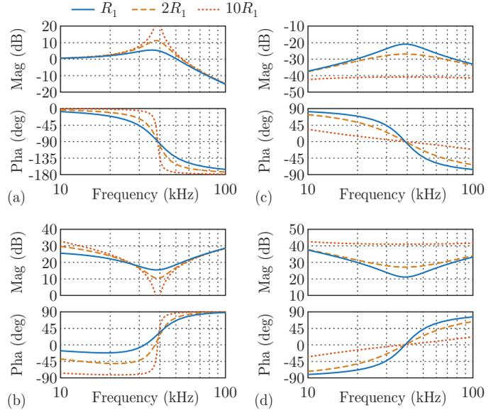
Fig. 5: Transfer function (a,c) and input impedance (b,d) Bode plots of the parallel (a,b) and the series (c,d) resonant converter depending on the equivalent resistance  $R_1$ .
