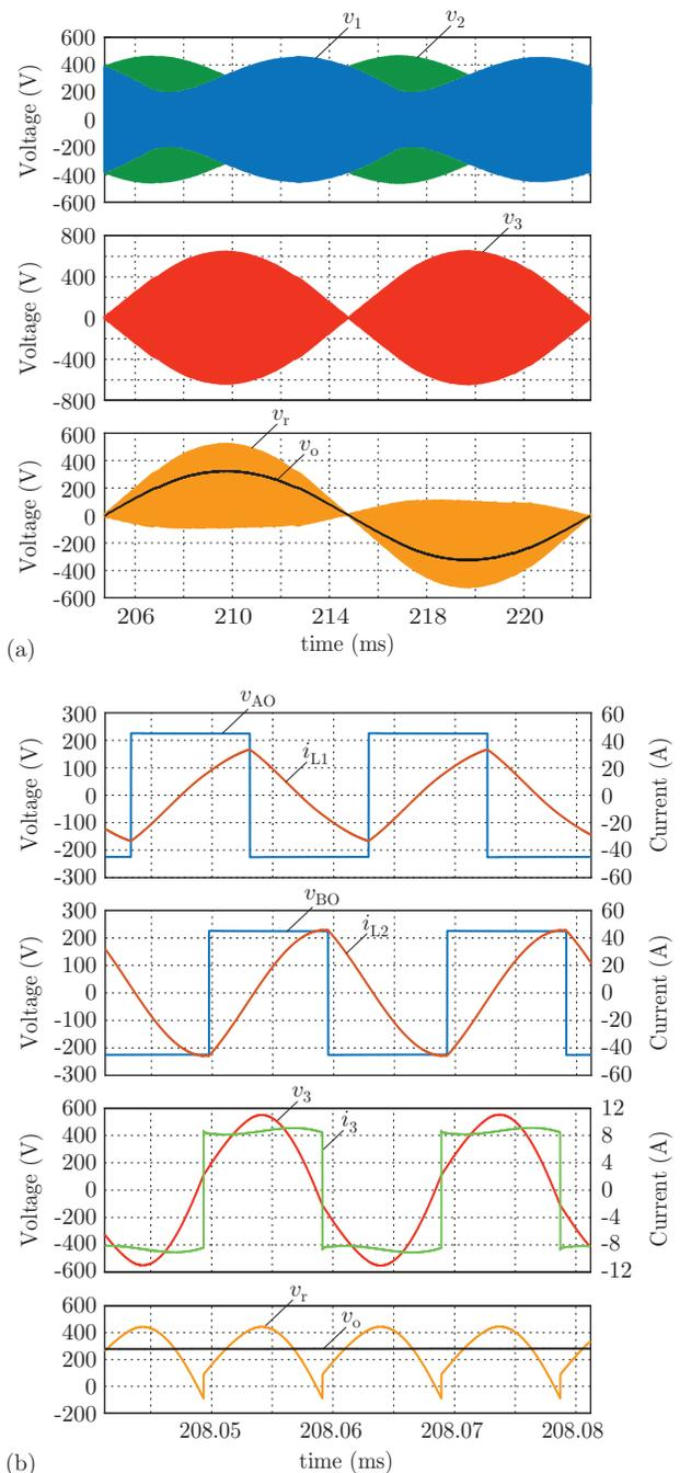
Fig. 7: Steady-state simulation results of the voltage-based SAM HF link inverter at rated output power for a mains period (a) and two resonant periods (b).
