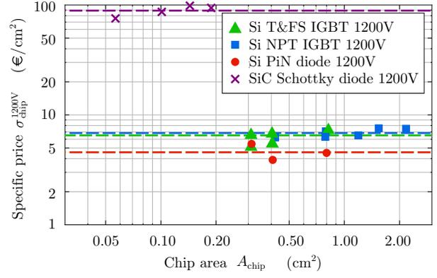
Fig. 3: Specific prices for common semiconductor chip technologies based on data from two major semiconductor manufacturers. The dashed lines represent the numerical values of the identified cost model parameters  $\sigma_{\text{chip},x}$  according to **Tab. I**.
