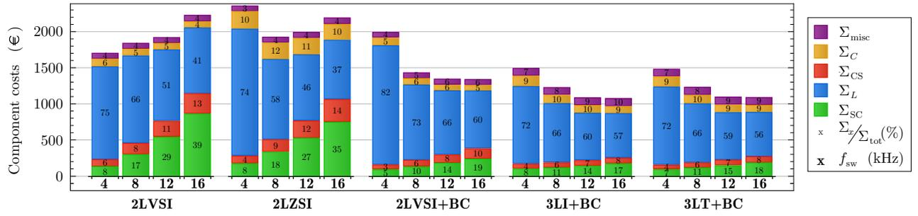
Fig. 9: Component cost structure per topology and switching frequency  $f_{sw}$ .  $\Sigma_{misc} = \Sigma_{PCB} + \Sigma_{IC}$  is the PCB and IC costs,  $\Sigma_C = \Sigma_{ELCO} + \Sigma_{film}$  the total capacitor cost and  $\Sigma_{CS} = \Sigma_{sink} + \Sigma_{fan}$  the cooling system cost. The output  $LCL$  filter is included in this analysis.
