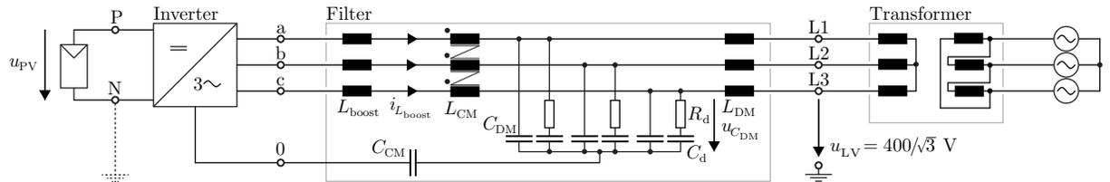
Fig. 7: Generic topology of the considered three-phase 50kW PV inverter with output LCL filter. A  $\Delta$ -Y transformer connects the 400V industrial low voltage secondary grid side to a European 50Hz medium voltage grid.
