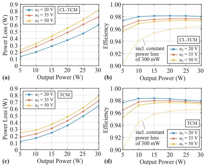
Figure 9: (a)-(b) Measured power loss and DC-DC efficiency of the CL-TCM converter at variable output power and different output voltages. (c)-(d) Measured converter performance with TCM operation. Note that these measurements do not include the constant power loss of the DSP/FPGA board.
