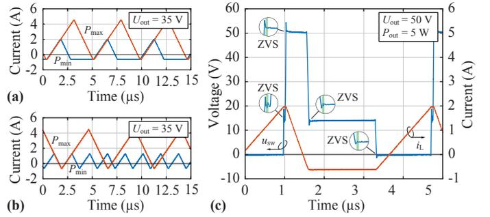
Figure 7: (a)-(b) Measured inductor current waveforms of the prototype converter in CL-TCM operation and TCM mode respectively. (c) Measured CL-TCM converter switch-node voltage  $u_{\text{sw}}$  and inductor current  $i_L$  indicating ZVS operation.
