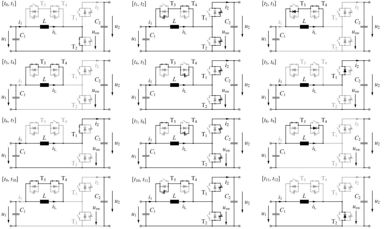
Figure 2: Operating states of the proposed ZVS modulation scheme for a full switching cycle  $[t_0, t_{12}]$ .
