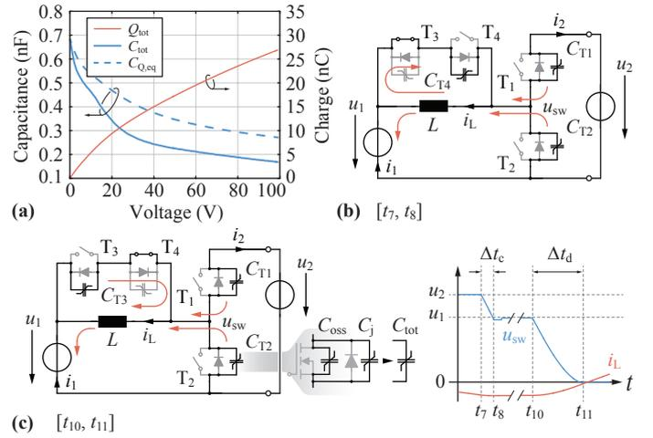
Figure 4: (a) Total switch output capacitance, charge-equivalent capacitance and stored charge. (b) Illustration of the current flow during the resonant voltage transition in time interval  $[t_7, t_8]$  and (c) in time interval  $[t_{10}, t_{11}]$ .
