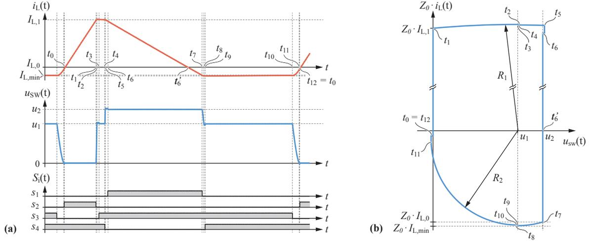
Figure 3: (a) Typical waveforms of the inductor current  $i_L$  and switch-node voltage  $u_{sw}$  and the switching states  $t_1$  to  $t_{12}$ . (b)  $u$ - $Z$ - $i$ -diagram, showing the scaled inductor current  $Z_0 i_L(t)$  with respect to the switch-node voltage  $u_{sw}(t)$ .
