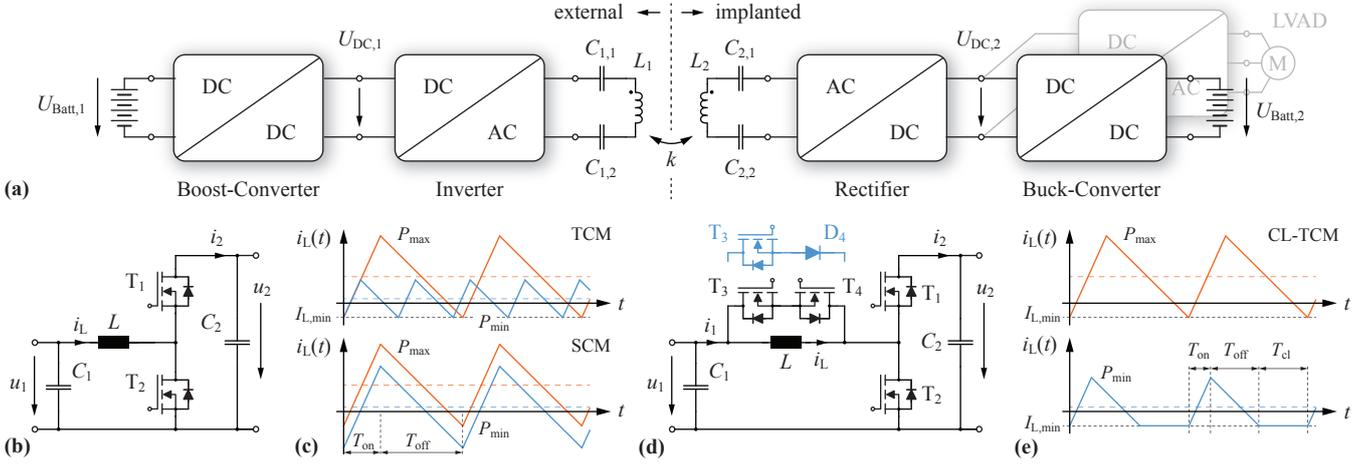
Figure 1: (a) Basic power management concept of the Transcutaneous Energy Transfer (TET) system. (b) Standard boost converter topology and (c) the inductor waveforms for Synchronous Conduction Mode (SCM) and Triangular Current Mode (TCM) operation. (d) Clamp-Switch TCM (CL-TCM) boost converter topology and (e) the associated inductor current waveforms.
