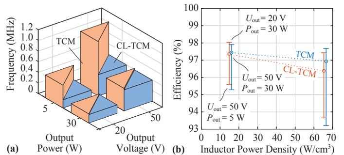
Figure 10: (a) Measured switching frequency variation of the CL-TCM and TCM converter with the inductor shown in Fig. 6(c). (b) Measured DC-DC efficiency of the CL-TCM and TCM converter with respect to the power density of the two inductors shown in Fig. 6(b) and (c). Note that the efficiency does not include the power losses of the DSP/FPGA board.
