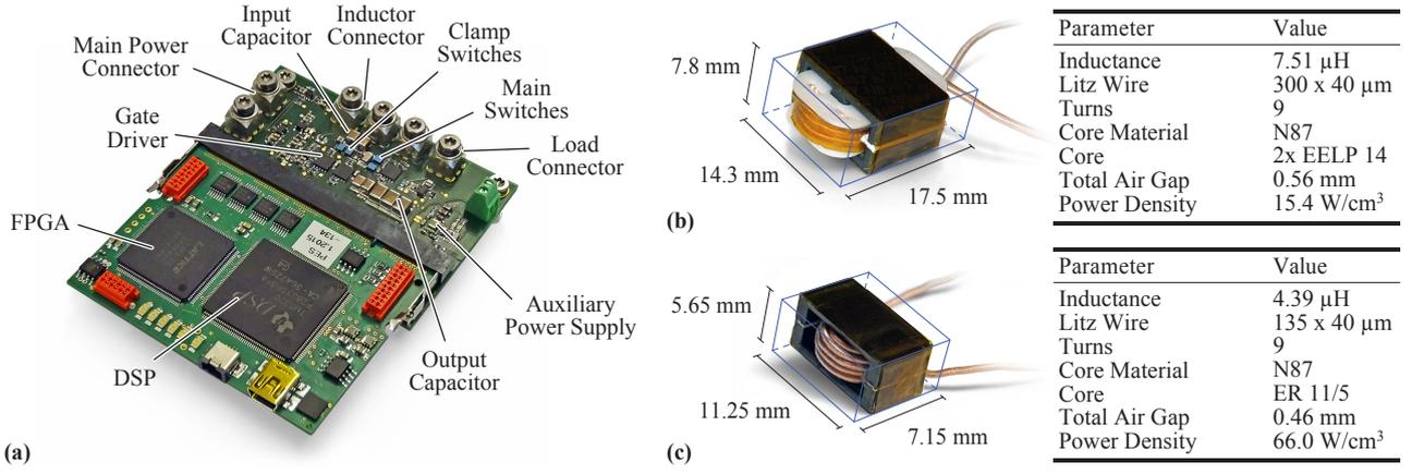
Figure 6: (a) Hardware prototype of the CL-TCM converter including the control board. (b-c) Realization and technical specifications of the inductors used for the performance evaluation of the CL-TCM converter.
