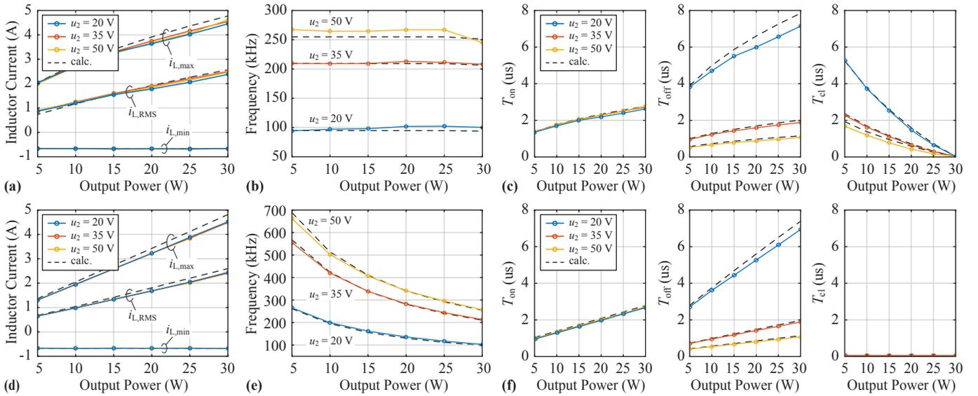
Figure 8: (a) Measured and calculated minimum, maximum and RMS inductor current values of the prototype CL-TCM converter. (b) Measured and calculated switching frequency and (c) on-, off- and clamping-time intervals of the CL-TCM converter. (d)-(f) show the same parameter measured for the converter operated in TCM mode.
