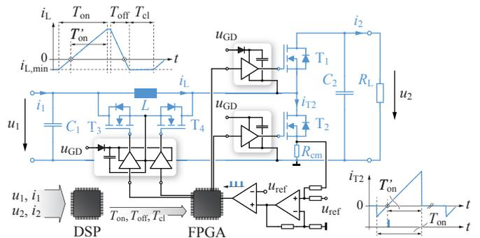
Figure 5: Realization of the control structure and recommended implementation of the inductor current zero crossing detection using a current measurement resistor at the low-side switch  $T_2$ .
