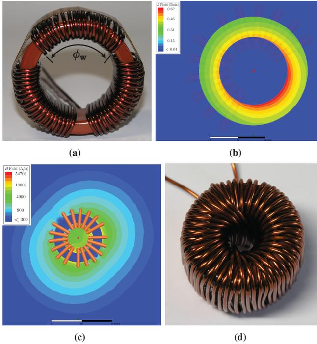
Figure 6. Representative 3-phase CM choke (a); flux density distribution in (b) and magnetic field distribution around (c) the CM choke's core as given in Table III for  $i_a = 30.0 \text{ A} + 135 \text{ mA}$  and  $i_b = i_c = -15.0 \text{ A} + 135 \text{ mA}$ ; and DM inductor realized with a toroidal core (d).
