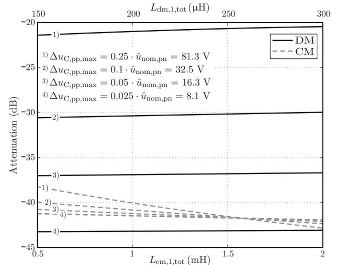
Figure 5. Achieved DM and CM attenuations of the first filter stage over  $L_{dm,1,tot}$  and  $L_{cm,1,tot}$ , respectively (cf. **Fig. 3**), for different DM as well as CM maximum peak-to-peak voltage ripples  $\Delta u_{C,dm,1,pp,max}$  and  $\Delta u_{C,cm,1,pp,max}$ . In the figure,  $\Delta u_{C,pp,max} = \Delta u_{C,dm,1,pp,max} = \Delta u_{C,cm,1,pp,max}$  is set.
