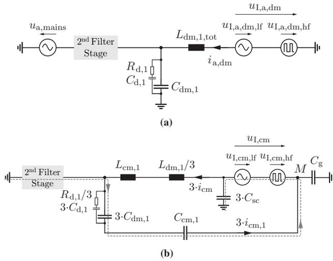
Figure 3. DM equivalent circuit (a) and CM equivalent circuit (b) of the bidirectional PWM rectifier system (cf. Fig. 1 and Fig. 2). The damping elements  $C_{d,1}$  and  $R_{d,1}$  are however neglected in the optimization.
