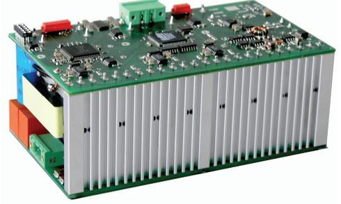
Fig. 11: Laboratory prototype of the ultra efficient and ultra compact 3kW TCM resonant-transition PFC rectifier with the specifications and components given in Table II. Dimensions: 137 $\times$ 56 $\times$ 78mm<sup>3</sup>, power density: 5kW/dm<sup>3</sup>, efficiency  $\approx$  98.3%.
