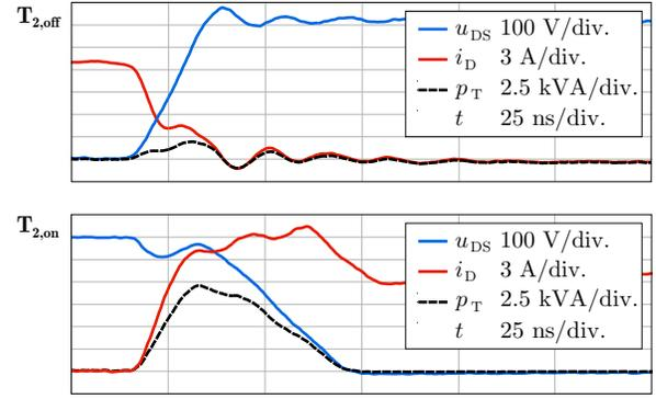
**Fig. 5:** Measured turn-off and turn-on switching loss energies  $E_{off}$ ,  $E_{on}$  respectively, for the commutation between one of the selected SiC JFETs and the internal body diode of the opposed JFET in the inverter stage of the 2LVSI+2LBC topology ( $I_D = 13$  A,  $U_{DS} = 600$  V,  $T_j = 25$  °C). It can be seen that the turn-off switching transition is close to zero voltage switching (ZVS).
