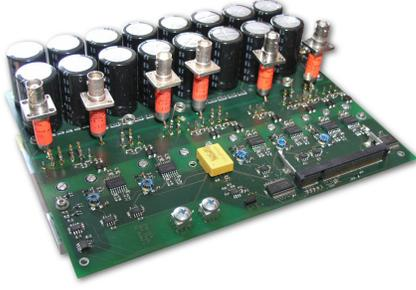
**Fig. 4:** Switching loss measurement test bench implementing a single phase bridge of the inverter stage of each topology.
