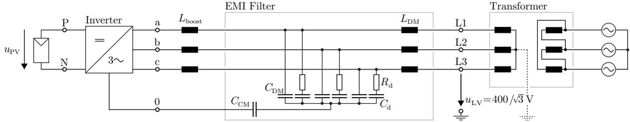
**Fig. 2:** Generic topology of the considered three-phase PV inverter with boost inductors and output  $LC$  EMI filter. A  $\Delta$ -Y transformer connects the 400 V low voltage secondary side (non-public industrial grid) to a European 50 Hz medium voltage grid. With minor adoptions in the filter due to different applicable EMI emission limits [6], the same topology could also be used in a (grounded) public low voltage grid.
