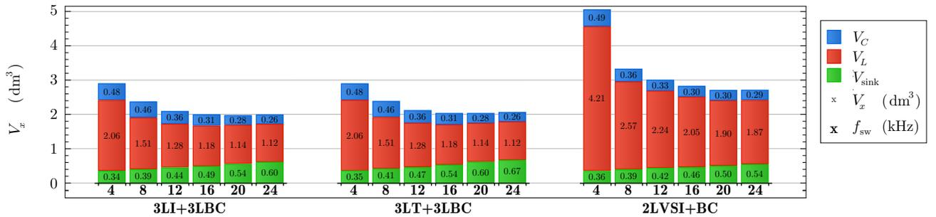
**Fig. 7:** Volume breakdown of the employed components for different switching frequencies  $f_{\text{sw}}$ .  $V_C$  is the total capacitor volume,  $V_L$  the total inductor volume and  $V_{\text{sink}}$  the volume of the required heatsink.
