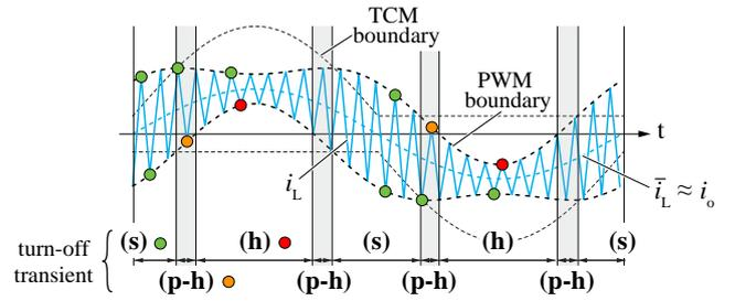
**Fig. 6:** Schematic inductor current waveform for PWM modulation if a rather small inductor value is selected. Due to the high current ripple, around the current zero crossings soft-switching (s) or at least partial hard-switching (p-h) can be achieved during turn-on. Hard-switching (h) only occurs if the lower current boundary gets positive. During turn-off always soft-switching is achieved.
