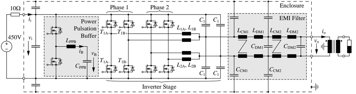
**Fig. 1:** Topology of the realized inverter consisting of two output phases, each of which is formed by two interleaved bridge legs in buck-configuration and a subsequent EMI output filter realized with two Common and Differential Mode (CM/DM) filter stages. The system DC-side energy storage is realized with an active Power Pulsation Buffer (PPB) [16].
