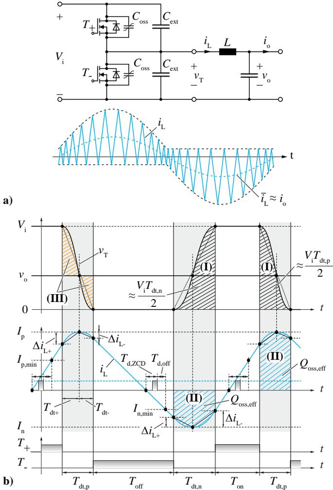
**Fig. 4:** Detailed explanation of challenges with defining the switching instances of the TCM modulation considering time delays of the ZCD and the gate drives ( $T_{d,ZCD}$ ,  $T_{d,off}$ ), **a)** bridge-leg with external capacitors  $C_{ext}$  placed in parallel to the MOSFETs in order to reduce the switching losses [7], **b)** detailed analysis of one TCM switching cycle.
