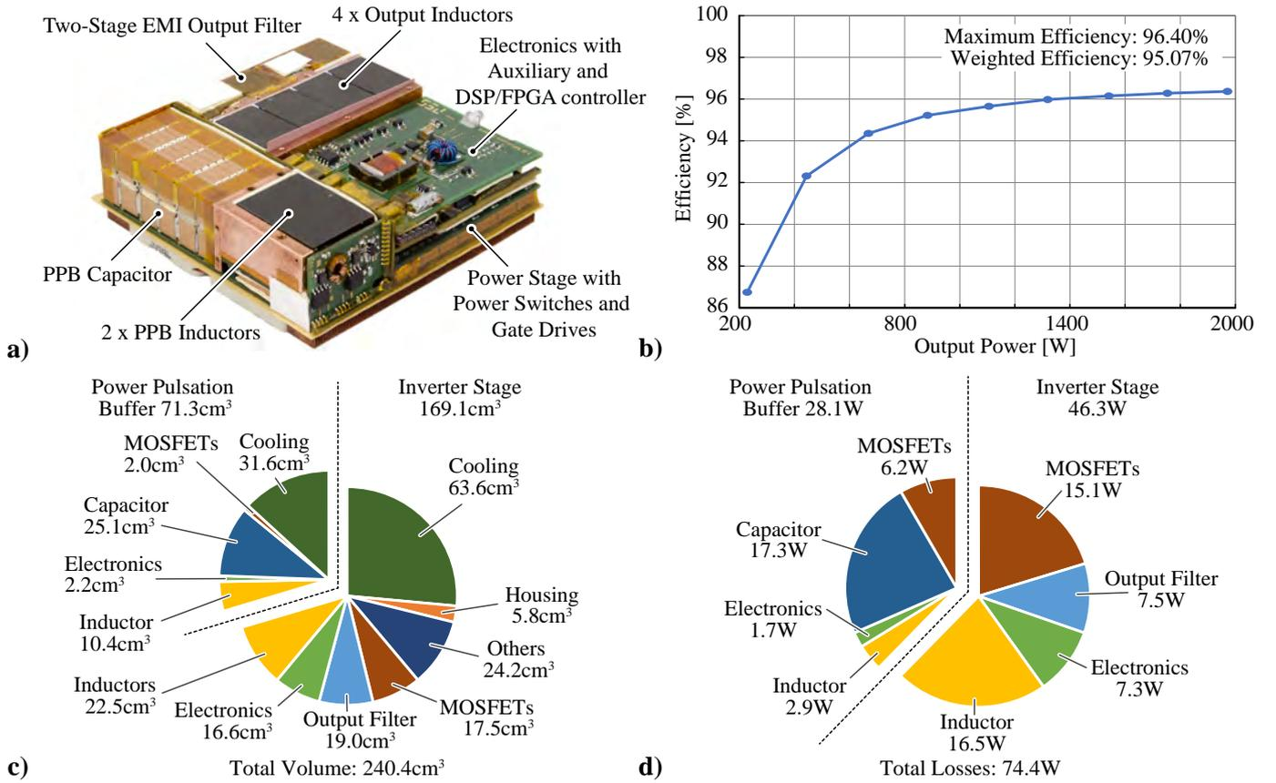
**Fig. 2:** a) Photograph of the realized hardware (without housing and top-side heat sink) presented by a team of ETH Zurich (PES), FH-IZM, and Fraza company, at the finals of the GOOGLE Little Box Challenge (3 cm x 8.8 cm x 8.9 cm), b) measured efficiency dependency on the output power, c) corresponding volume distribution and d) loss distribution.
