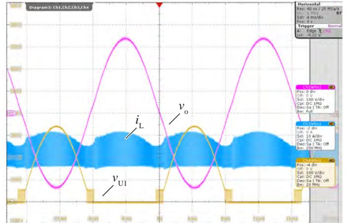
**Fig. 9:** Measured waveforms of the proposed modulation strategy for the DC-AC Buck Converter & Unfold of **Fig. 7** at an output power of 1 kW. Inductor current  $i_L$  (10 A/div), bridge-leg voltage  $v_{U1}$  (100 V/div) and output voltage  $v_o$  (100 V/div).
