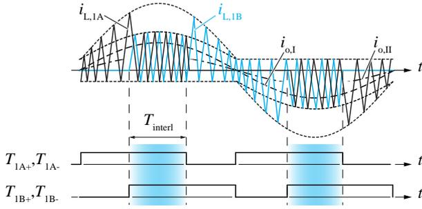
**Fig. 5:** Schematic current waveforms for the implemented 4D-Interleaving [25] in order to improve the converter efficiency, especially in the part load range. The duration  $T_{\text{interl}}$  of the time intervals in which both bridge-legs are interleaved, is adjusted depending on the actual output power.
