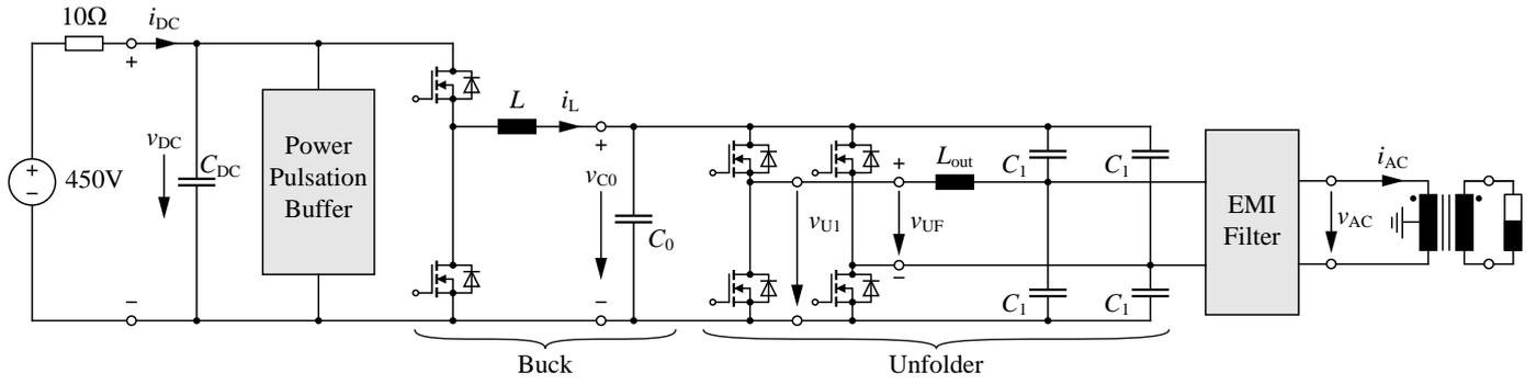
**Fig. 7:** Inverter topology based on a conventional buck converter and a subsequent low-frequency full-bridge unfold.
