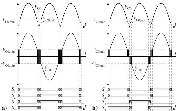
**Fig. 8:** Modulation strategies of the proposed control scheme where **a)** either both bridge legs are switched or **b)** only one bridge leg is operated with PWM and the other bridge leg is clamped.
