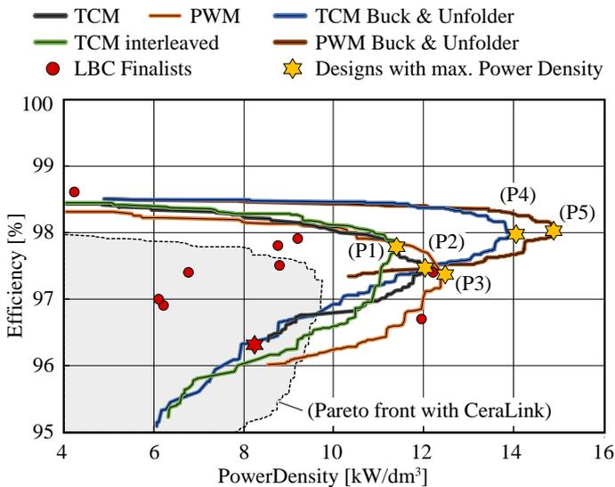
Fig. 12: Calculated Pareto fronts with respect to efficiency ( $\eta$ ) and power density ( $\rho$ ) of the described circuit topologies with different modulation schemes (TCM/PWM) and with/without interleaving of bridge-legs.
