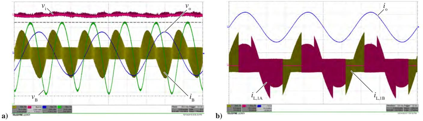
**Fig. 3:** **a)** DC input voltage  $v_i$  (2 V/div, AC-coupled), generated AC voltage  $v_o$  (200 V/div), PPB capacitor voltage  $v_B$  (20 V/div), and TCM current  $i_B$  in the PPB inductor (10 A/div), **b)** output current  $i_o$  (10 A/div) and corresponding TCM currents  $i_{L,1A}$ ,  $i_{L,1B}$  (10 A/div) in the interleaved half-bridges of one output phase, whereas in the vicinity of the current zero-crossings only a single bridge-leg is operated alternately (4D-interleaving [25]).
