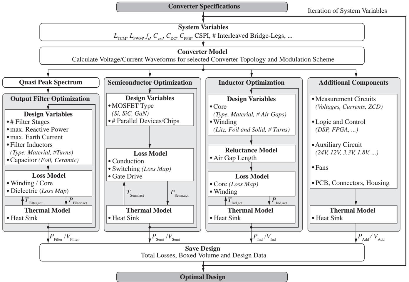
**Fig. 10:** Flow chart of the  $\eta\rho$ -Pareto optimization procedure.
