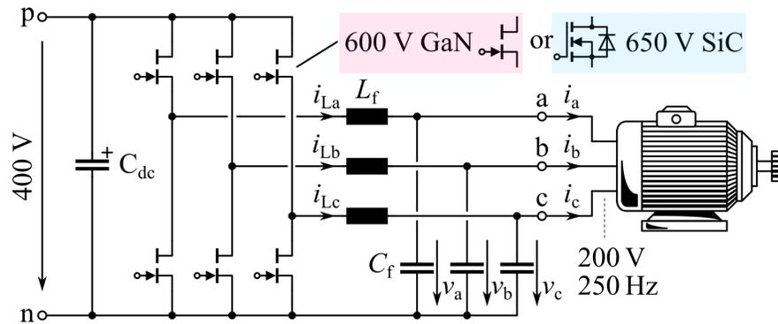
Specs: 2.5 kW inverter / 3-hp motor
