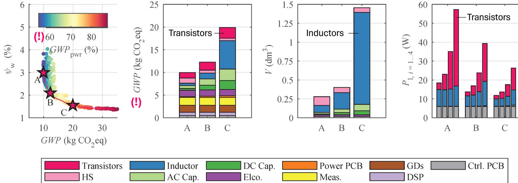
■ **Auxiliary electronics limit min. GWP (!)** — Similar: housing, etc. (not considered) — Dep. on rated power!
