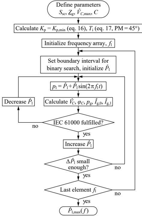
Fig. 9. Flow chart of the procedure to determine the maximum available load power at the PFC's output without violating IEC 61000. The maximum feasible power for a predefined set of distinct frequencies is determined by means of a binary search algorithm. An ohmic AC load is assumed, i.e.,  $\hat{P}_1 = P_0$ ; still, any other relation between  $\hat{P}_1$  and  $P_0$  could be used.
