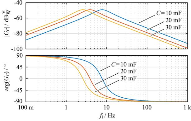
Fig. 7. Disturbance transfer function of the PFC rectifier,  $\underline{G}_C$ , for three different DC-link capacitances. Since the proportional gain of the PI controller is the same for all three cases, also the maximum values of the disturbance transfer functions are of same value.
