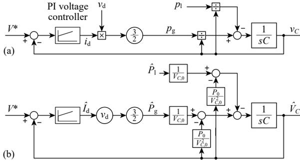
Fig. 6. (a) LF large-signal and (b) small-signal models of the PFC rectifier in the synchronous  $dq$  reference frame, for operation with defined load power.
