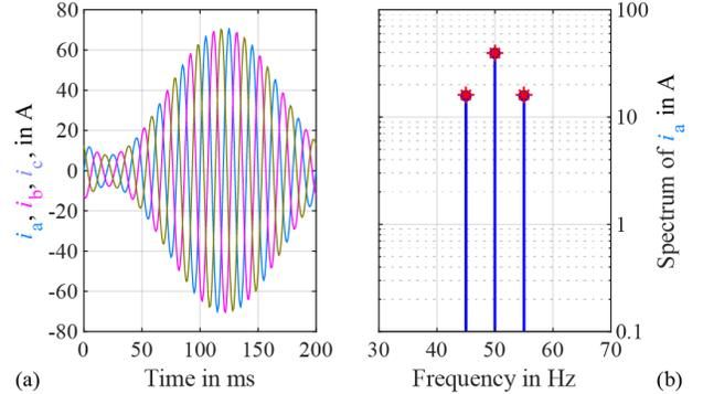
Fig. 3. (a) Simulated grid-side phase currents and (b) corresponding amplitude spectrum of each phase (same spectra result for all three phases; blue: simulation, red stars: calculation with (9)). The shown results consider operation according to (5), i.e., DC-link voltage and instantaneous power waveforms of Fig. 2 apply. The common envelope of the phase currents is directly proportional to  $p_g(t)$ , since the amplitudes of the grid voltages are assumed to be constant.
