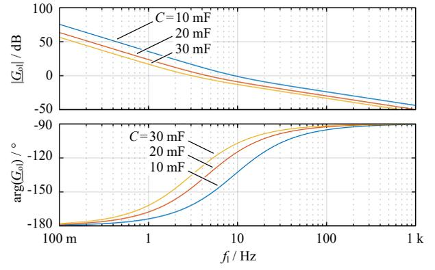
Fig. 8. Open-loop transfer functions of the PFC rectifier,  $\underline{G}_{ol}$ , for  $K_p = K_{p,\min}$ , a phase margin of  $45^\circ$ , the specifications listed in Tab. I, and three different capacitance values,  $C = \{10 \text{ mF}, 20 \text{ mF}, 30 \text{ mF}\}$ .
