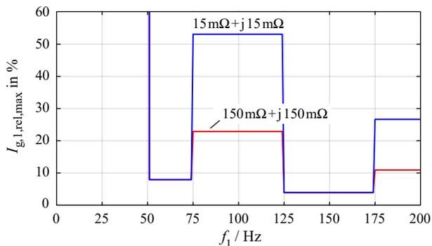
Fig. 4. Frequency characteristic of the maximum allowable sideband amplitudes of the grid currents to comply with IEC 61000-3-12 (grid current harmonics) and shown for two different grid impedances. The amplitudes are given as percentages of the frequency component at mains frequency,  $\hat{I}_{g,0}$ , which is proportional to the average output power, i.e.,  $\hat{I}_{g,0} = 2 P_0 / (3 v_d)$ .
