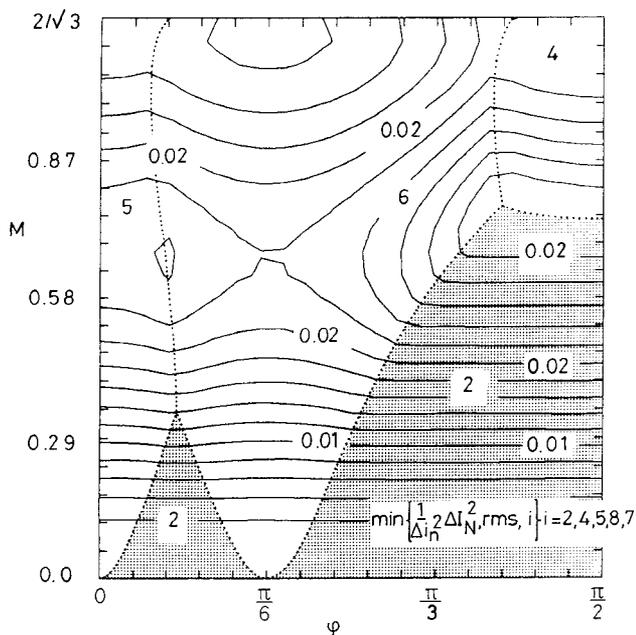
**Fig.3** Application regions of the different modulation methods for minimum harmonic losses,  $\min\{1/(\Delta i_n^2) \Delta I_{N,rms,k}^2\}$   $k=2,4,5,6,7$  (continuous modulation 2 and discontinuous modulations 4, 5, 6 or 7)
