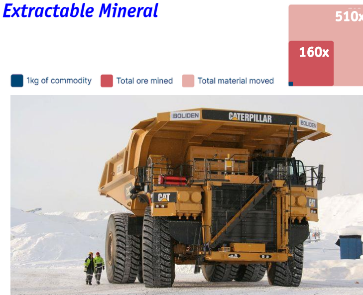
Caterpillar 797F — 350 tons payload / 3 MW
